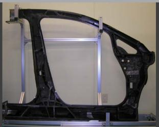
Ultimate Lightweight Aluminum/ **CFRP Body Side Panel by Topology**
