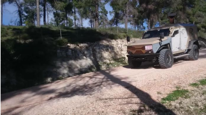
Irish Bridge Crossing Test, 45km/h
