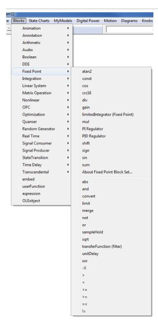
The 33 element VisSim EMBEDDED fixed point blockset ("Blocks/ Fixed Point") is used to design and simulate performance of fixed point algorithms prior to codegen and execution on an embedded platform.
