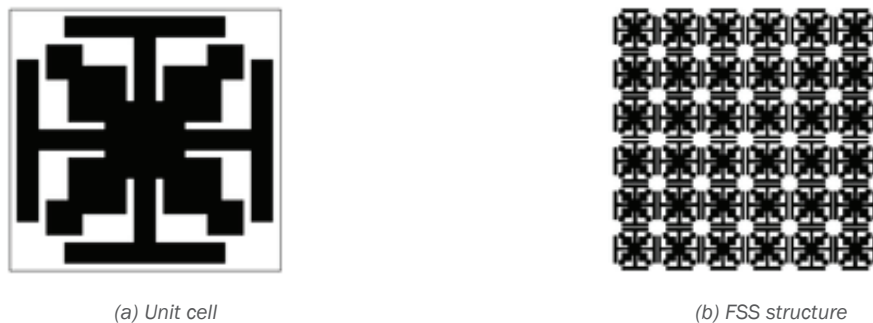
Figure 4: Combination of Jerusalem cross and three-step fractal patch
