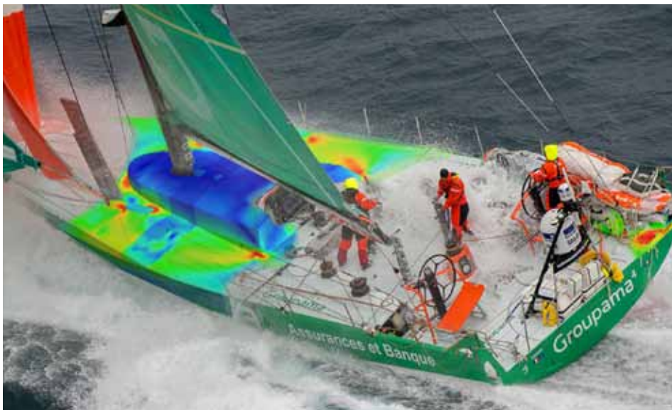
[AB]structures had to develop three structurally optimized but unique racing yachts in a preset time frame, considering the boundary conditions of the Volvo Ocean Race challenge.
