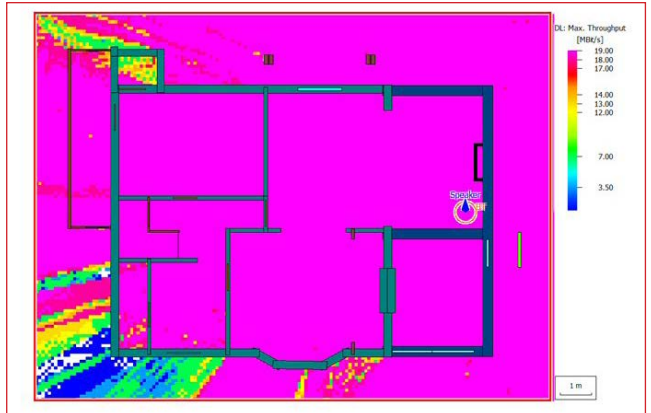
▲ Fig. 13 Maximum achievable DL throughput for the BT speaker.
