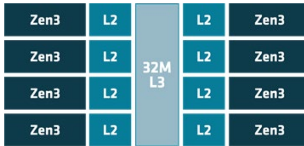
Figure 1 AMD EPYC 7003 Processor L3 Cache layout
