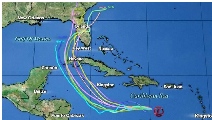
Figure 7: The precise initial conditions of a hurricane are unpredictable. Multiple simulations account for a collection of initial conditions (indicated by the red circle) and gives rise to multiple solutions based on which probabilistic forecasts of its trajectory are made
