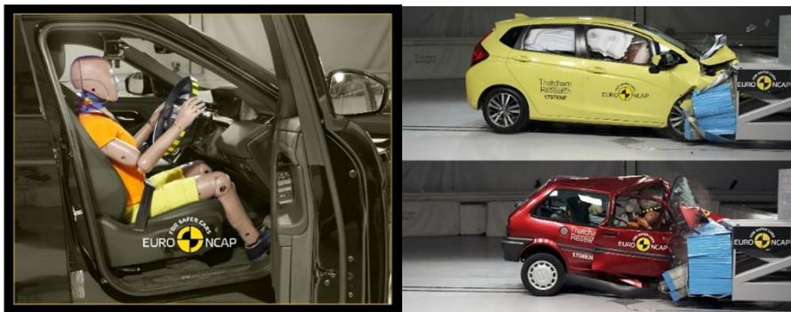
Figure 1 – Crash tests require carefully instrumented and calibrated test dummies, multiple vehicle prototypes, advanced, comprehensive sensing, and numerous repetitions. Simulations are a lower-cost alternative.
