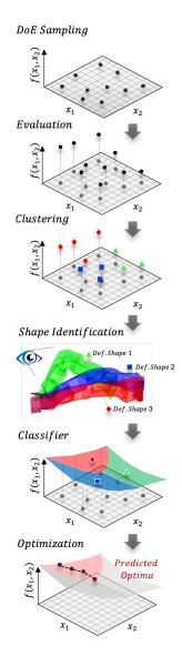
TOP: Front crash scenario, load paths in the car, deformation behavior of the longitudinal beam. RIGHT: The Expert **Emulation Optimization Process:** DoE Sampling, Evaluation, Clustering, Shape identification, Classification & Optimization
