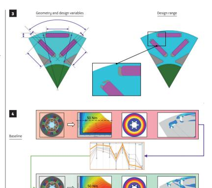
**3.** Simulation can be used to determine optimal location, orientation, and size of the rotor magnets
