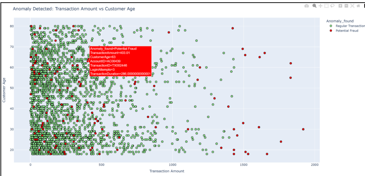
Figure 17 - Anomaly detection using Isolation Forest (PyOD): scatter plot visualization in AI Studio and Tooltip in Python plotly
