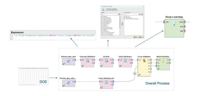
In Altair Al Studio, the optimization function is used to set certain proportions of data to conduct a reverse search for the optimal ratio of polyurethane adhesives and adjustable process parameters.
