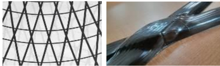
Fig. 3. Example of displaced overlapped node
