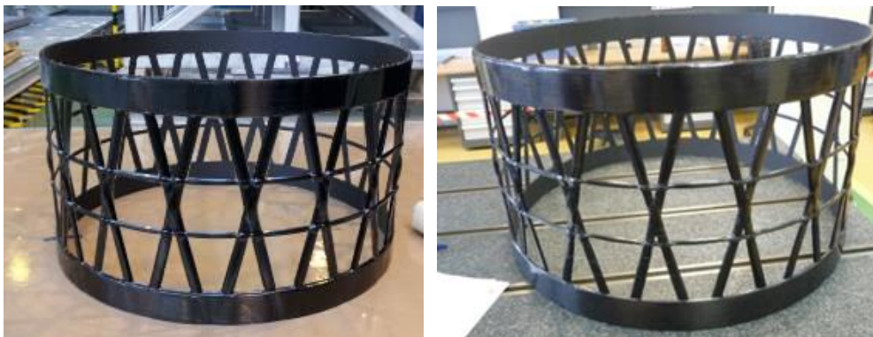
Fig. 7. Cylindrical demonstrators HM fibre (left), UHM fibre (right)
