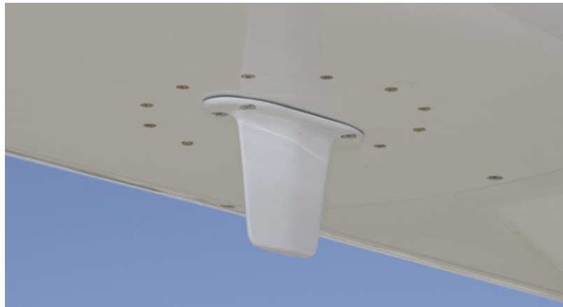
Figure 2 – A typical blade antenna mounted on the fuselage of the aircraft.
