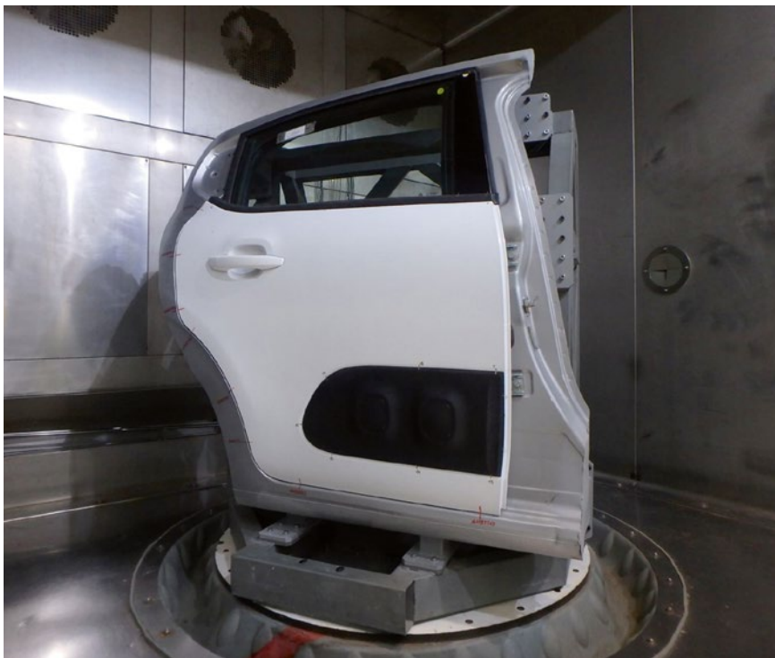
FIGURE 1 S&R physical testing on interior assemblies (© PSA)
