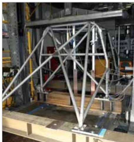
Instrumentation of roll cage with sensors and strain gauges for measurement of deflection and strain
