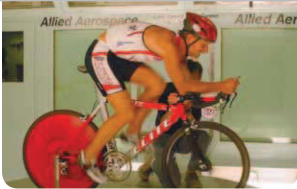
Zipp Speed Weaponry, a manufacturer of advanced bicycle racing wheels, couples wind tunnel testing with the use of computational fluid dynamics software to assess design options.
