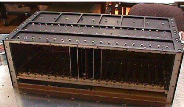
Fig. 1 CAD model (top) and the EQM model of ADPMS aluminium housing
