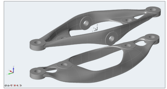
Altair Inspire screenshot of optimized parts. The number of unique components could be significantly reduced.
