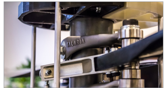
The topology optimization of the rotor hubs resulted in a weight reduction of almost 30%.
