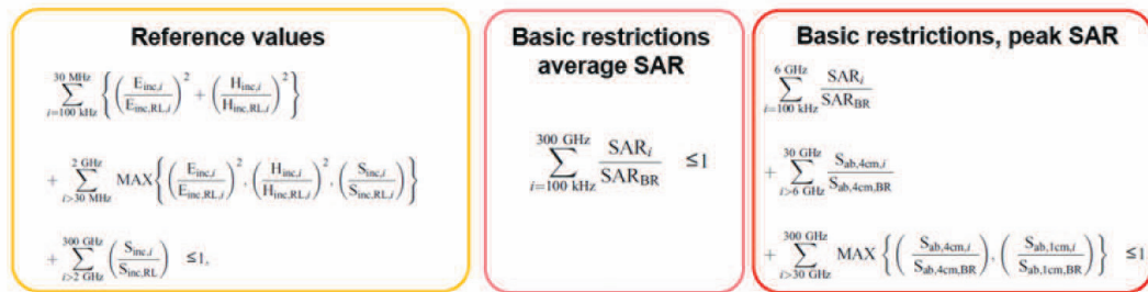
Figure 7: Summation formulas for evaluation of RADHAZ exposure to multiple frequencies
