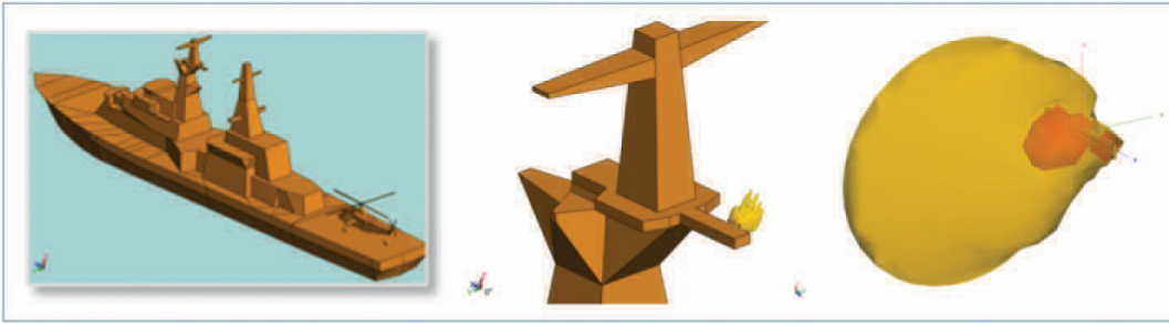
Figure 9: RADHAZ zone simulation for a scanning radar mounted on a ship
