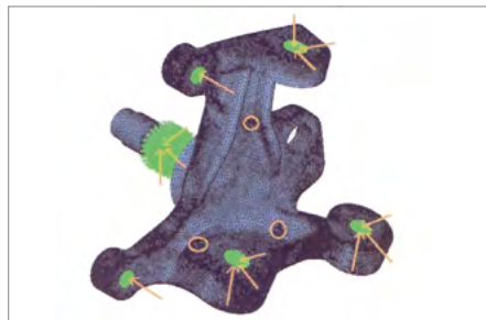
Load case combination of steering, braking, and bumping.
