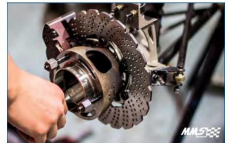
The new titanium upright was designed to be interchangeable with the existing aluminum upright.
