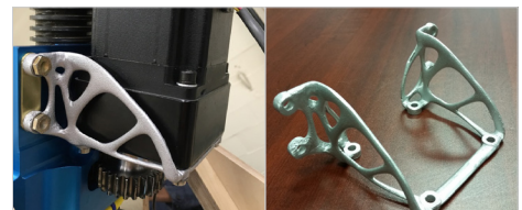
New Bracket Produced with Additive Manufacturing in use
