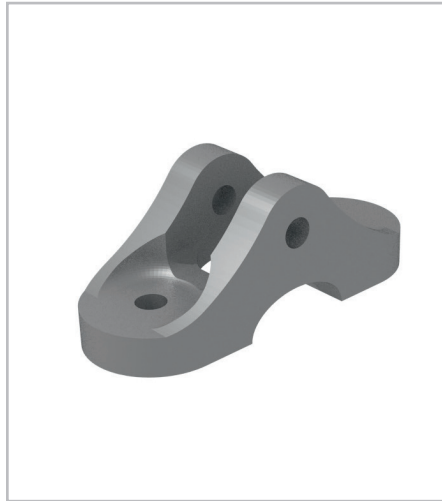
The Titanium brackets have been optimized by starting with the definition of the design and the non-design space. The succeeding topology optimization revealed different possible designs from which the final form (center picture) was selected and then virtually tested in a finite element analysis.
