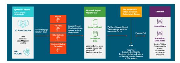
Monarch and Monarch Server provide highly accurate, multi-layered pattern recognition, data extraction, and data preparation capabilities in a versatile, no-code development environment. The software is agnostic about data formats and sources and can capture data from virtually any source, including PDF, text, and XML files, along with any SQL database and the most common big data sources.
