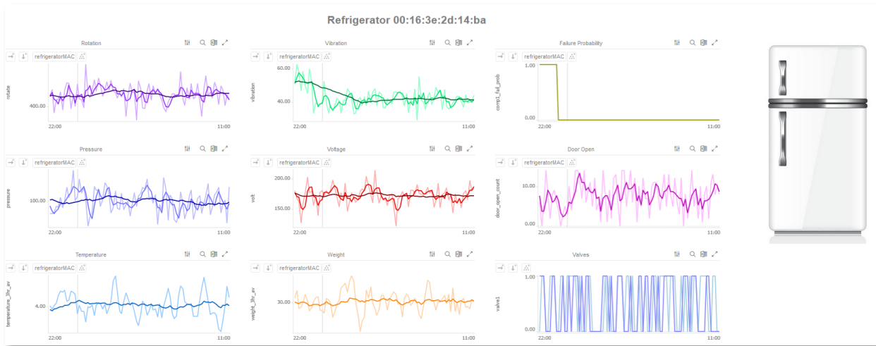
Figure 20 – Final visual dashboard with the sensor data and the failure probabilities from the predictive model.
