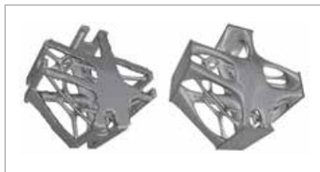
OptiStruct topology optimization (density distribution at different iteration steps) and HyperWorks mesh output (standard (left), and smoothed final design (right) of the connecting node structure.
