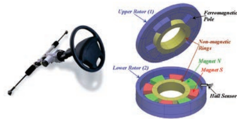
Position sensor designed in Flux 3D
