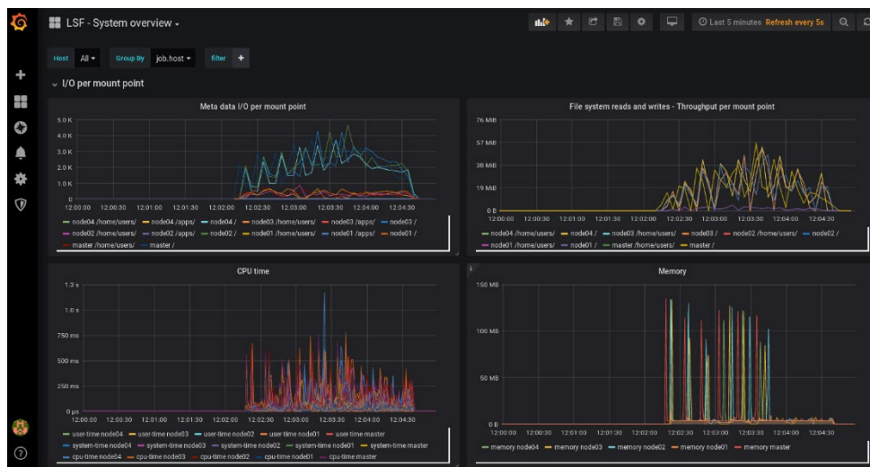
Normal I/O: Mistral data tracking per-job metadata, bandwidth, CPU, and memory
