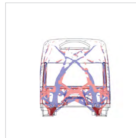
Visualization of tensile (red) and compressive (blue) stresses
