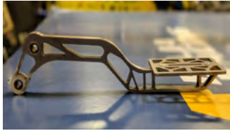
LEFT: 2019 vehicle mid-turn in the Tennessee maneuverability event. Awarded 1st place in every maneuverability course in the 2019 season. TOP: Team photo at the 2020 vehicle unveiling. This car sports an all new four-wheel drive system developed to conform with the new 2021 rules. BOTTOM: 2017 brake pedal. Analyzed and optimized via OptiStruct.
