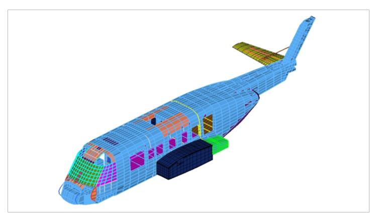
A finite element solver, by Michigan Engineering Services (MES), suitable for mid to high frequency vibro-acoustic simulations. EFEA calculates structural vibration and interior noise using a small number of finite elements.
