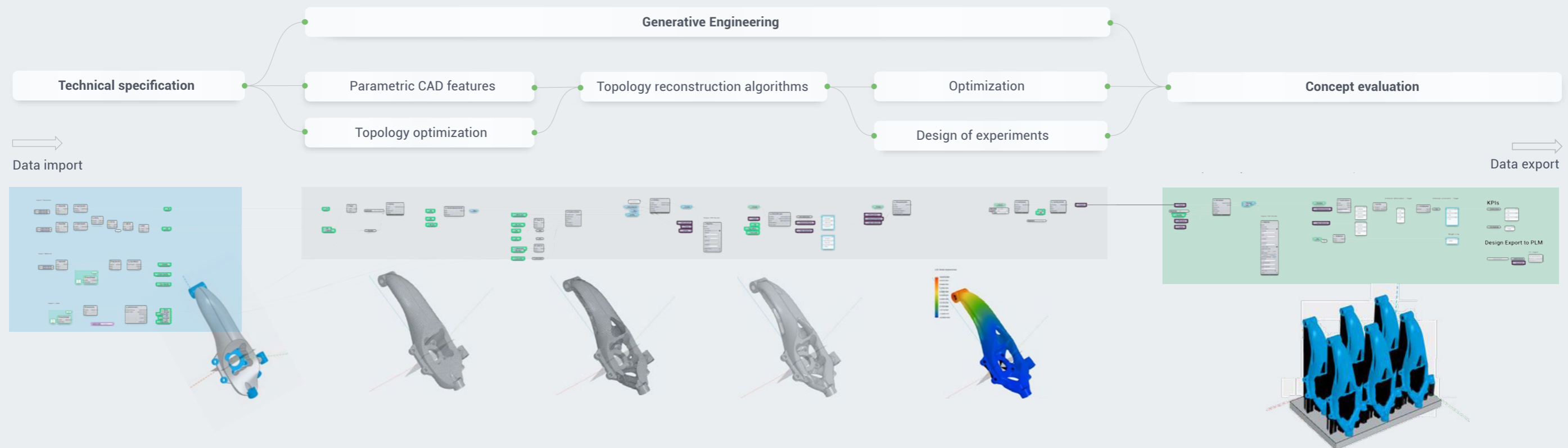
Figure 2: Technical DNA of a steering knuckle; from technical specification, generative features to concept evaluation
