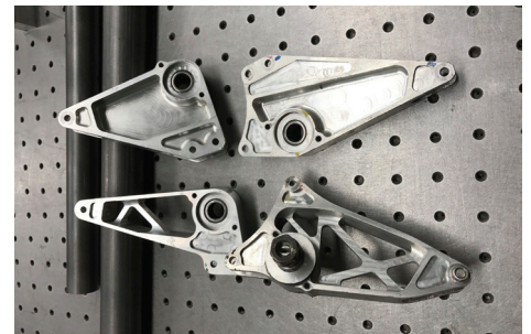
Redesigned bell crank compared to old bell crank
