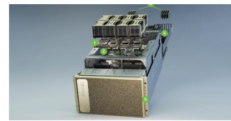
The NVIDIA DGX A100 system includes 8 GPUs, 6 NVIDIA NVSwitches, 10 Mellanox network interfaces, dual 64-core AMD CPUs, 2TB system memory, and 30TB Gen4 NVMe SSD
