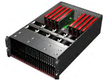
NEC SX-Aurora TSUBASA rackserver with 8 tightly integrated Vector Engines
