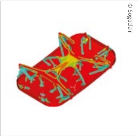
Altair Inspire: Topology Optimization of the EOLE access door
