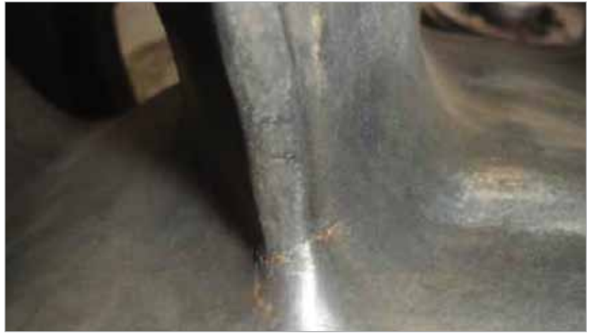
Die failed at the root of the shunting bridge after extruding more than 100 billets.
