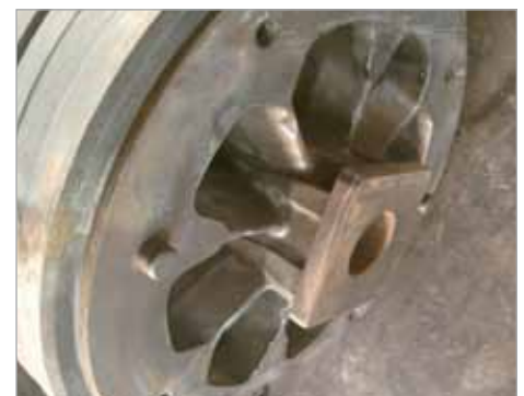
The second design had a much longer production life and was able to extrude more than 10 tons of the alloy.
