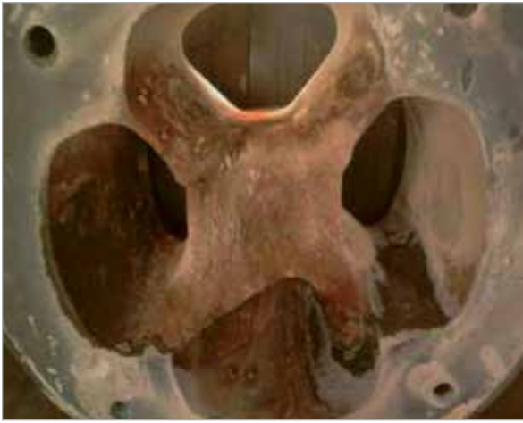
Mandrel cracked in the bridge region as predicted by the HyperXtrude analysis.
