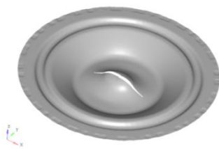
Fig. 8 Crack propagation with element deletion at forming limit
