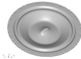
Fig. 15 Crack propagation with MMC fracture model
