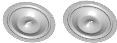
Fig. 16 From left to right, crack propagation without and with XFEM method.
