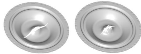
Fig. 17 From left to right, crack propagation using a MMC criterion and using a NXT criterion
