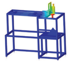
LEFT: Machine's X, Y & Z axis final result after design change. TOP: Machine's X axis results at initial design stage. MIDDLE: Machine's Y axis results at initial design stage. BOTTOM: Machine's Z axis results at initial design stage.
