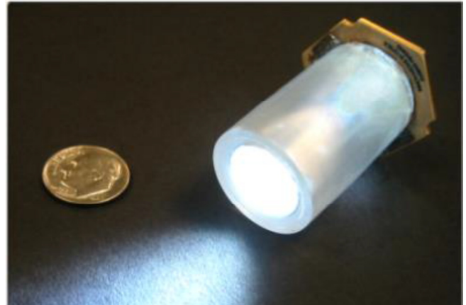
Hybrid design with non-imaging optic to shape emission
