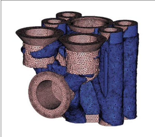
Fig. 2 Generating the valve block shape with OptiStruct
