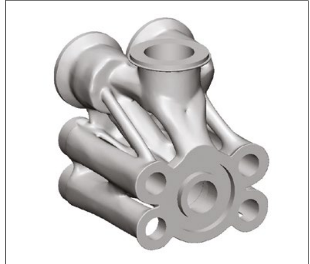
Fig. 3 Smoothing of the geometry with 3-maticsSTL to prepare model for Additive Manufacturing
