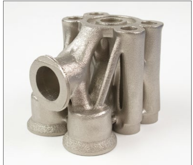
Fig. 7 The additively manufactured valve block
