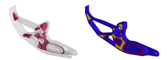
4. **Calculate material strength/hardness** – I assume that it is well-known that material strength in all materials depends on wall thickness but the decisive factor is solidification velocity. Solidification time can be observed and material strength and hardness can be calculated to compare how they are influenced by different methods.
