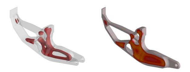
3. Investigate where defects related to solidification can appear – The size of these defects is also very interesting because most times it is impossible to achieve a sound casting, but it is desirable to achieve defect-free areas and as small defects as possible in the remaining areas of the casting. Defects can be exported from the simulation software as 3D models for use as input data e.g. in further calculations.
