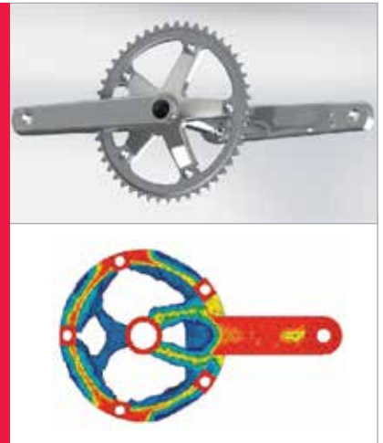
Top: Original bicycle crank design Bottom: Topology optimization result
