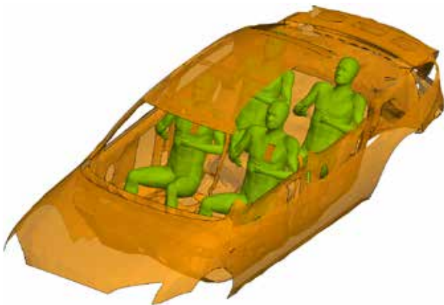
SAR computation for phantoms wearing personal radios in a vehicle
