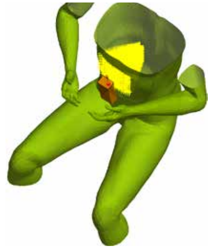
Phantom with radio close to body
