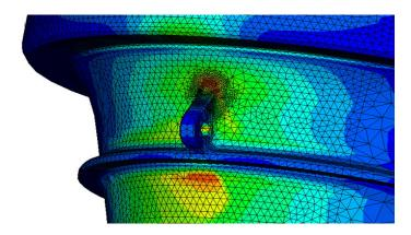
"Our Mills are dynamically severely loaded. S-Life enables us to conduct a comprehensive strength assessment and component optimization in a simple and fast way. The program also facilitates the documentation of the analysis."
