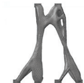
TOP: Comparison between initial optimization results and final design, resulting in a 54% weight saving compared to the existing part.
