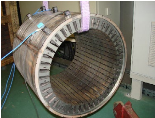
IkerMAQ internal test points. Red: K-thermocouples; Blue: Magnetic test coils
