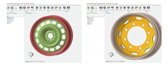
LEFT: Using the custom solution developed within HyperWorks, Accuride engineers were able to mesh complex parts, like the model with over 160k elements shown here, in minutes. **RIGHT:** Several FE modeling parameters – including element size, quality, and meshing techniques – can be controlled within the HyperWorks workflow.
