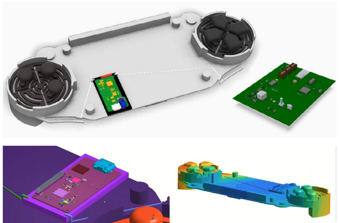
Structural analysis of game controller and PCB with Altair SimSolid.
